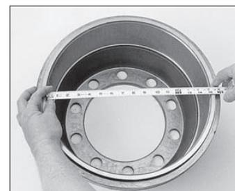
1. Braking surface diameter
